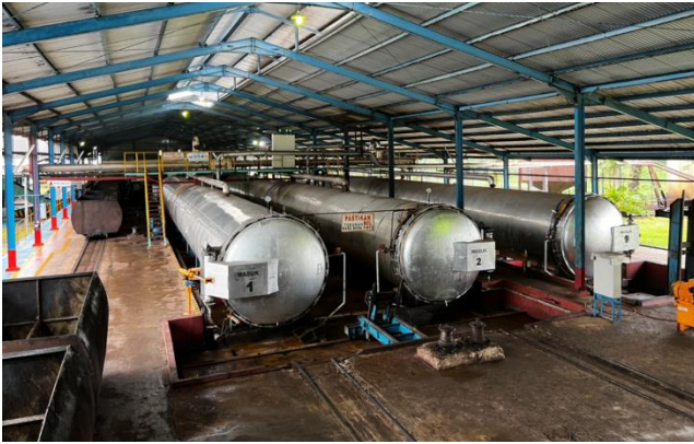
Fig 15. FFB boiling process in palm oil mills before...
