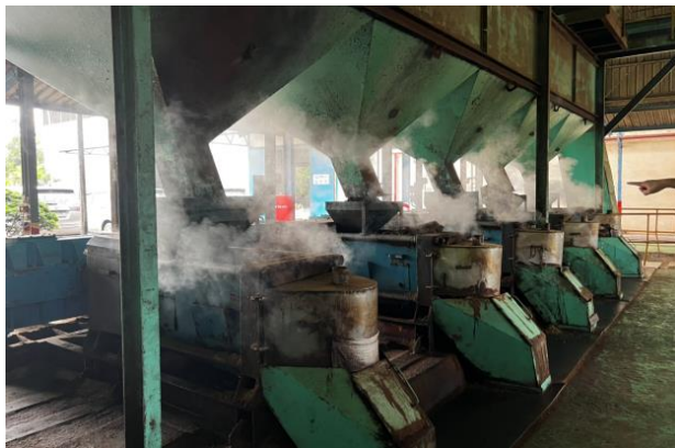
Fig 17. Palm kernel plant producing palm kernel oil...
